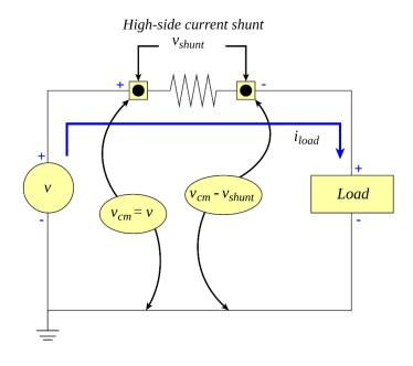
In this example, if you wanted to measure the current going to a load in a 12VDC automotive system, the easiest way *may* be to measure the battery feed, as many times the case of the device is grounded to the chassis. So you would need an isolated differential input (like the RAD-IO2-AIN), or at least an A/D that has a common mode well over the feed voltage (up to 18 VDC to be safe)
