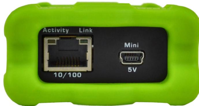
**Figure 2: RAD-Moon Conventional Ethernet Side.** Left, the standard Ethernet RJ-45 jack with integrated *Link* and *Activity* LEDs; right, a mini-USB jack that provides power to the device.
