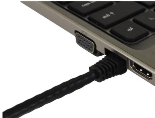
Figure 8: Connecting the Ethernet Cable to a PC. You can also connect it to an Ethernet switch, hub or other standard Ethernet device.
