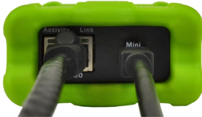
Figure 9: Connecting the Ethernet Cable to the RAD-Moon.
