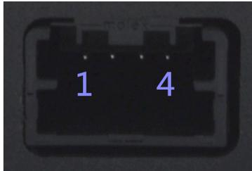
Figure 4: RAD-Moon BroadR-Reach Mini50 Jack with Pin Numbers. Pins are numbered 1 to 4 from left to right looking at the jack, as shown.
