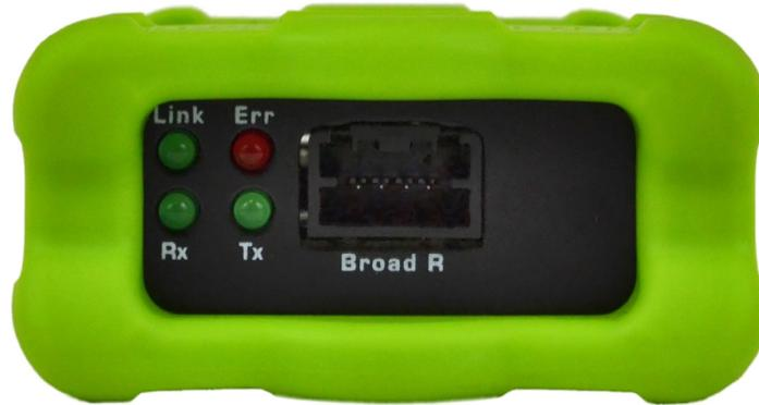
**Figure 3: RAD-Moon Automotive Ethernet Side.** The Mini50 BroadR-Reach connector can be seen here in the center, with the bank of status LEDs to the left.
