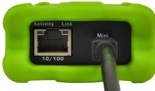
Figure 7: Connecting the USB Cable to the RAD-Moon.
