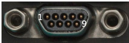
Figure 87: neoVI FIRE 2 μDB-9 Connector Pin Numbering.
