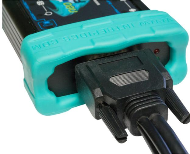
Figure 52: Connecting the HD-26 Cable Connector to the neoVI FIRE 2.
