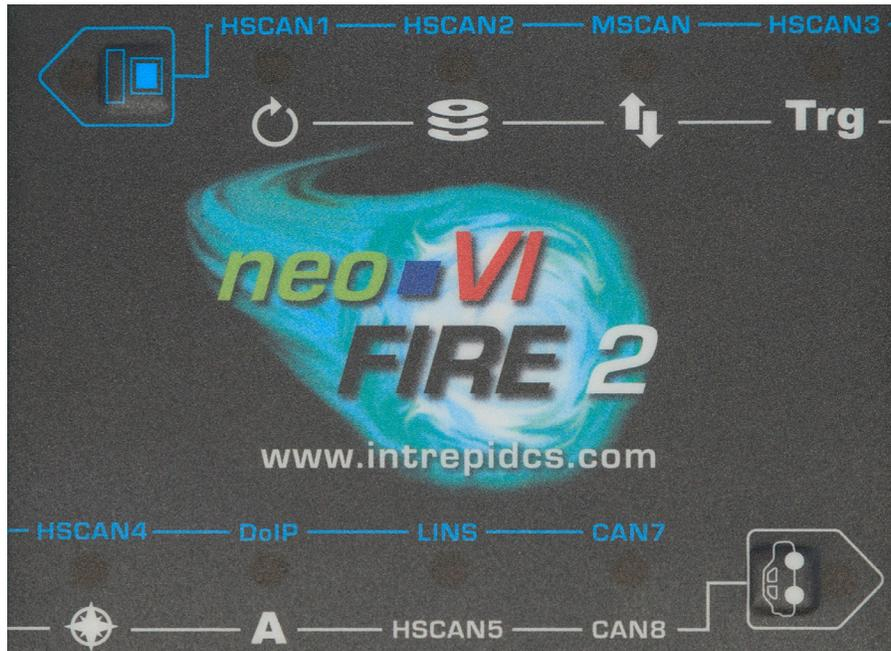
Figure 7: neoVI FIRE 2 Membrane LED Display and Keypad.
