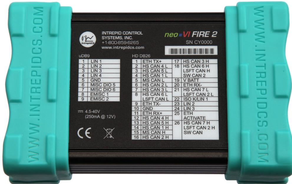
Figure 4: neoVI FIRE 2 Bottom View. Note that the FIRE 2's miscellaneous I/O channels are "EMISC 1" and "EMISC 2". (The "MISC DIO 5" and "MISC DIO 6" entries will be removed in future FIRE 2 label printings.)
