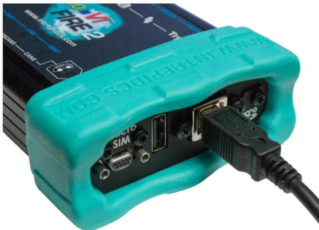
Figure 55: Connecting the USB Cable to the neoVI FIRE 2.
