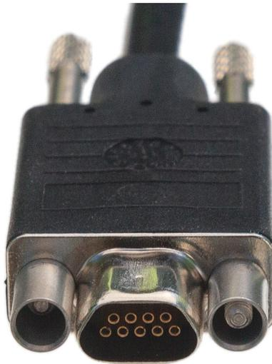
Figure 11: Close-up of  $\mu$ DB-9 Connector. This connector attaches to the mating connector on the neoVI FIRE 2, adapting it into an industry-standard DB-9 connector.
