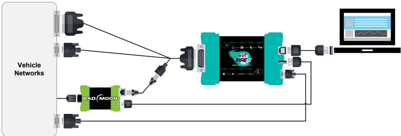
Figure 85: neoVI FIRE 2 Hookup Diagram for Automotive Ethernet Using RAD-Moon Media Converter.
