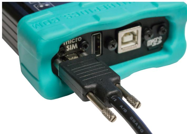
Figure 54: Connecting the μDB-9 Cable Connector to the neoVI FIRE 2.
